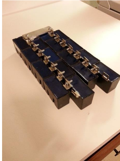
Figure 24: One 125nF capacitor bank
