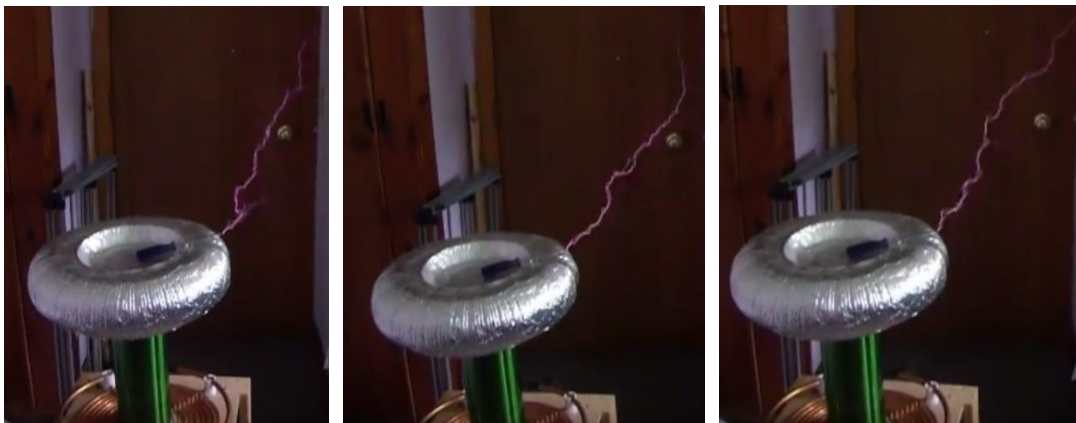
Figures 63-65: Slightly better tuning after doubling the tank capacitance
