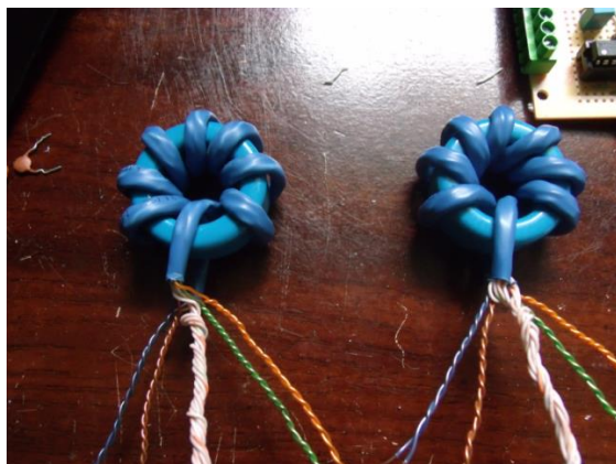
Figure 34: Gate drive transformers created using CAT-5 Ethernet cable
