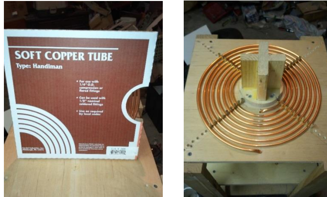
Figures 28 and 29: Pre-coiled copper tubing for use as the primary coil
