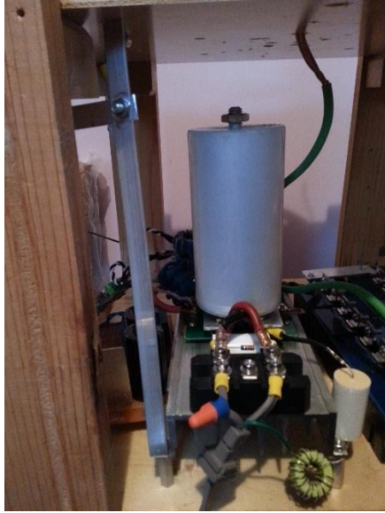
Figures 54 and 55: Aluminum grounding strap connected to RF ground
