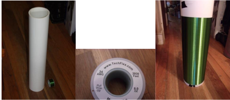
Figures 20, 21, and 22: Components that make up the secondary coil
