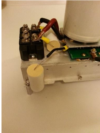
Figure 53: H-bridge assembly with primary strike protection capacitors installed
