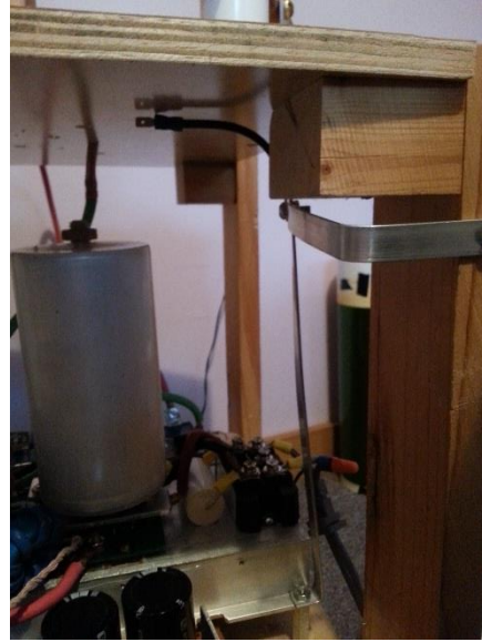
Figures 54 and 55: Aluminum grounding strap connected to RF ground
